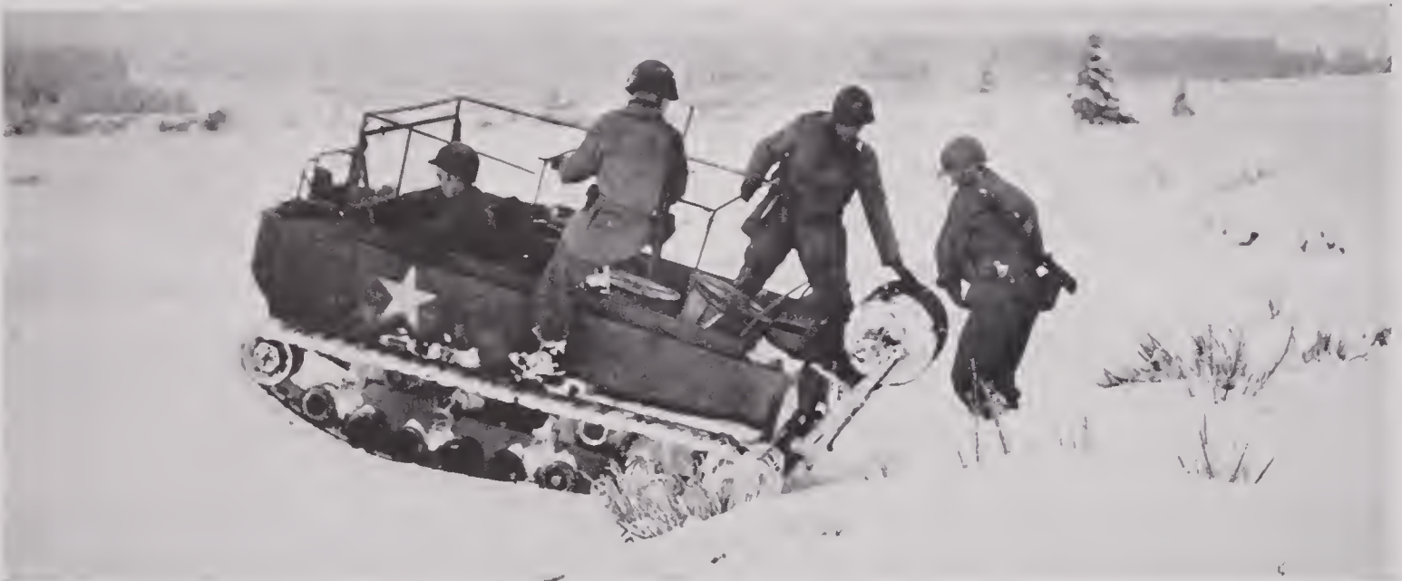
FIGURE 62. M-29 Weasel used for wire-laying operations in snow, European Theater of Operations.
